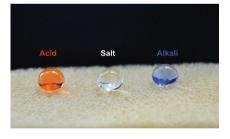
Inspired by superhydrophobic selfcleaning lotus leaves and porous biomaterials, polyurethane foam with simultaneous superhydrophobicity and superoleophilicity is fabricated. The resulting foam exhibits super-repellency towards corrosive liquids, self-cleaning, and oil/water separation properties, thus possessing multifunction integration.
